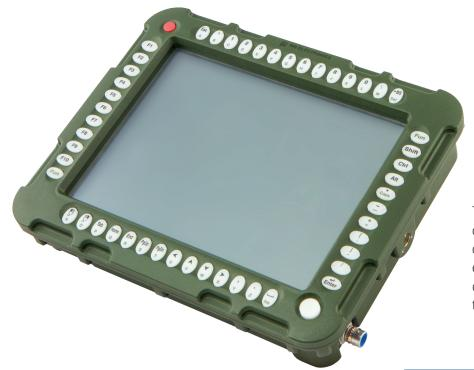
The design of the device ensures trouble-free operation in harsh operational environments of wheeled and tracked vehicles where the equipment is exposed to shocks, vibrations, dust, the wide range of humidity and ambient temperatures.
