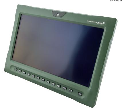
With the built-in standard FONET user interface and a headset connector, the terminal can be used as a part of FONET Digital Intercom System.
