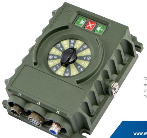
CZS-2FFS is also fitted with a 3-button keyboard which provides an emergency broadcast mode and an access to voice menu of settings (e.g. voice level).
