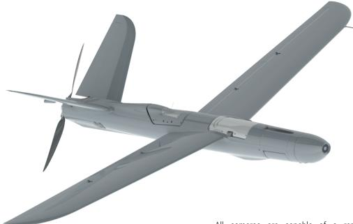
The reconnaissance version is based on the same fuselage and the ground segment as the WARMATE combat unmanned aerial vehicle – the observation payload and the warheads for combat missions can be used alternatively.
